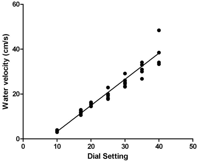
Figure A2. Change in water velocity measured by timing the movement of fluorescein in a fluid dynamics chamber
