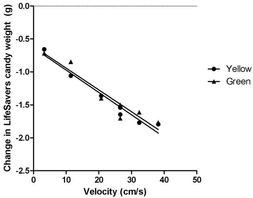
Figure A3. Change in weight of green and yellow LifeSavers™ candies calibrated using known water velocities in the fluid dynamics chamber
